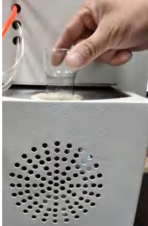
Figure 3-14 Installing a quartz burner tube
