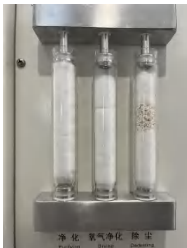
Figure 3-6 the reagent tube installation is finish
