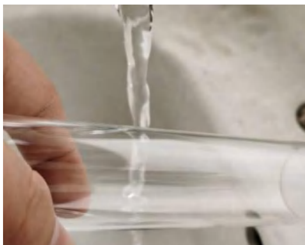
Figure1-6the quartz burning tube was cleaned with water
