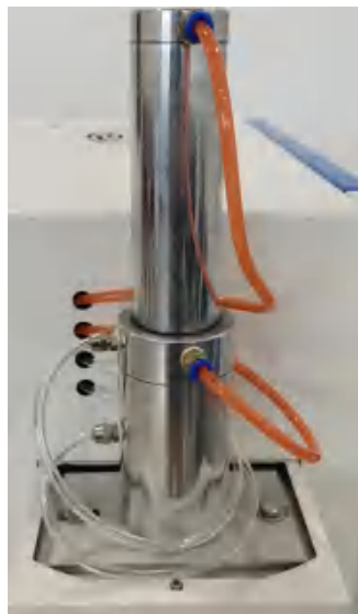
Figure 2-14make the Cleaning system install original position, and check gas line whether isn't connect right
