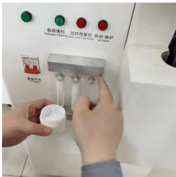
Figure 3-18 Applying vacuum silicone grease
