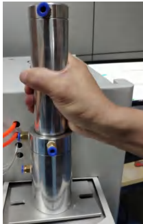
Figure 3-15 Installing the burner
