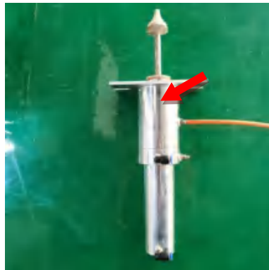
Figure 2-4 Cleaning the filter way
