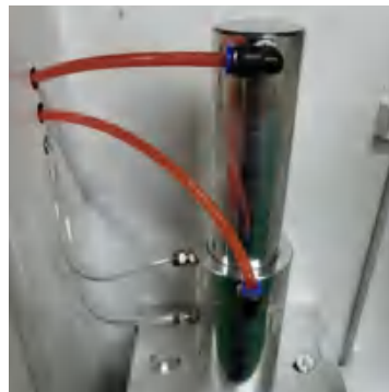
Figure 2-14make the Cleaning system install original position, and check gas line whether isn't connect right
