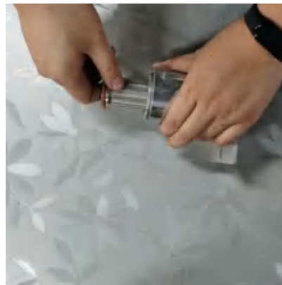
Figure 2-10 take the filter out
