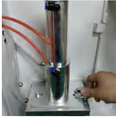
Figure 2-1 Pull out the Furnace head
