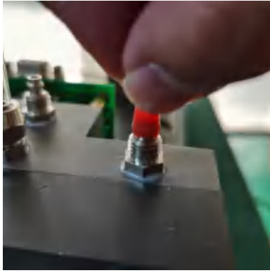
Figure 2-27 the Gas tube to connect to the interface
