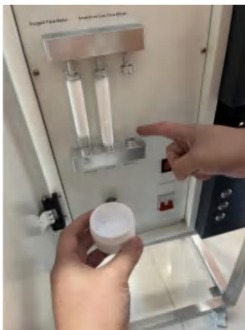
Figure 3-17 Applying vacuum silicone grease
