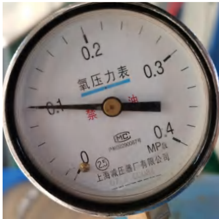
Figure 2-26 adjust valve to 0.1Mpa
