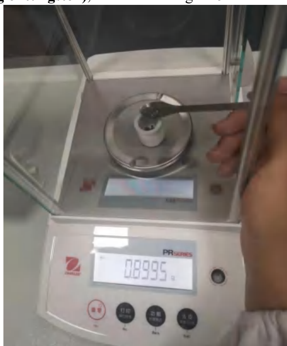
Figure 5-4 Adding tungsten particles
