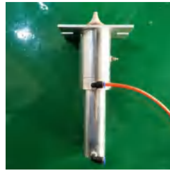
Figure 2-13 when the gas tube to connect to main pole pack up automatically
