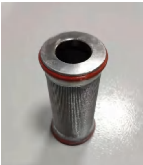
Figure 2-11 after the filter cleaned
