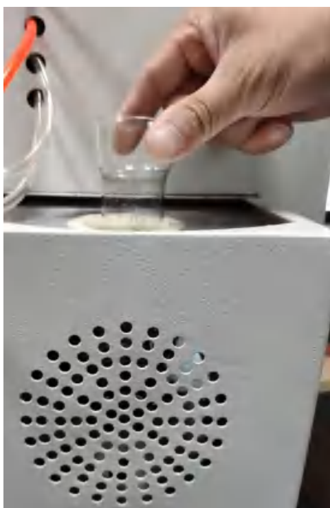
Figure 3-13 Installing a quartz burner tube
