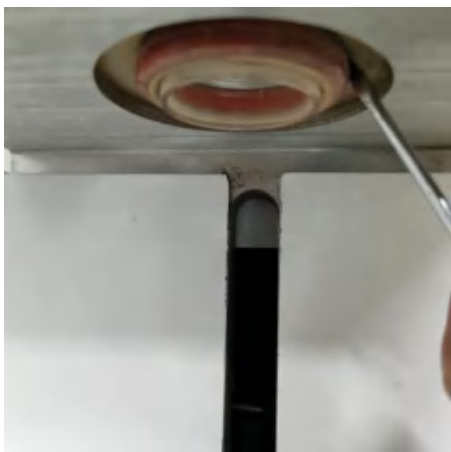
Figure1-3 remove the “O” type sealing ring
