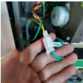
Figure 2-22 remove the white interface
