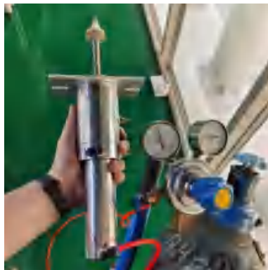
Figure 2-3 adjust reducing valve
