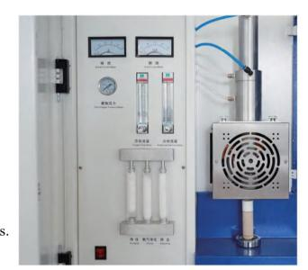
10. The system of high-frequency combustion and infrared detection system adopt fiber connection, cutting off direct electrical connection between the two, avoiding the burning furnace or external circuit can produce interference by cable transfers to infrared monitoring system
