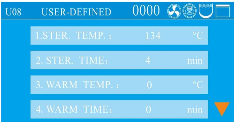
Press SET/ENT button to start modification, when the words are blinking, press UP or DOWN button to change the value, press SET/ENT again to confirm the modification, then press DATA to save and exit.
