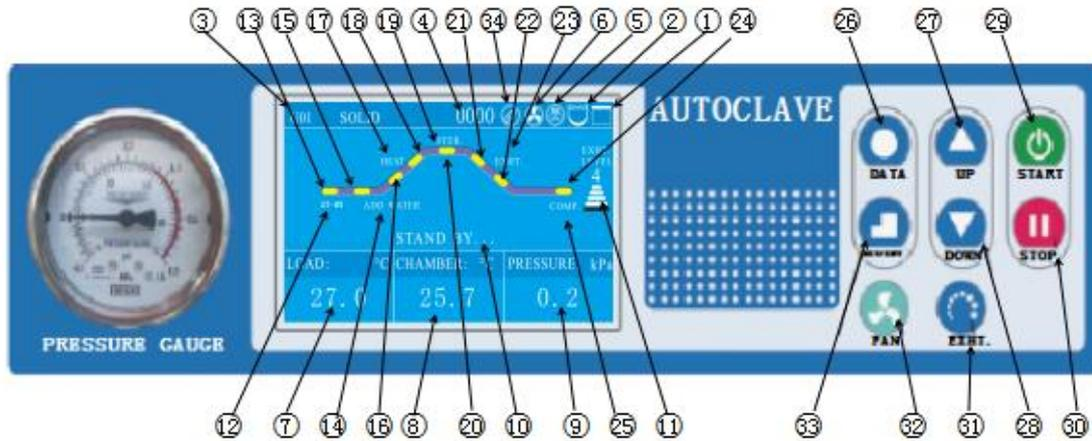
1.Lid interlocking icon:White when lid closed and locked, white and blinking when lid closed but not locked,red and blinking when lid is not closed.
