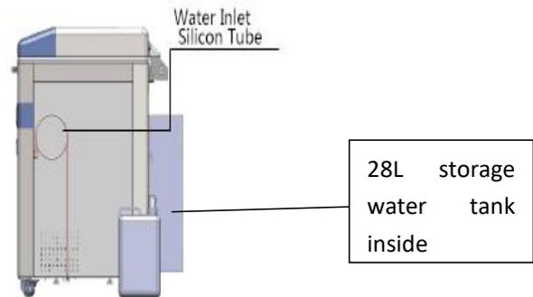
● If the water level of the back storage water tank drops below the LOW mark, a flashing icon “
