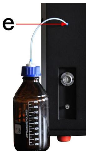
e. Solvent recovery port connected with PTFE pipe and solvent recovery bottle
