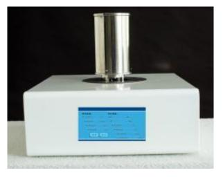
DSC: melting, crystallization, phase change, reaction temperature and reaction heat, combustion heat, specific heat...
