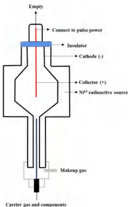
Figure1-9 Schematic diagram of ECD structure
