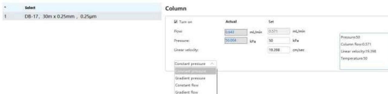
Figure 3-15 Chromatographic column method edit window
