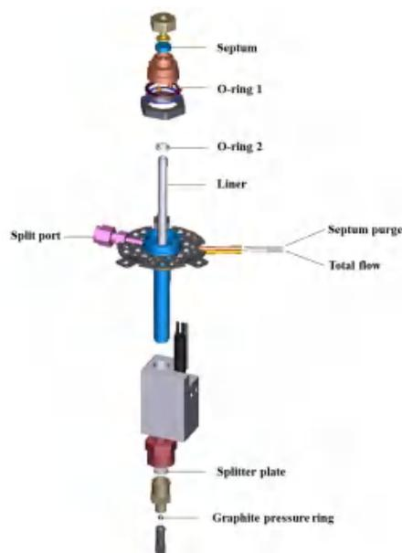
Figure 4-1 Inlet structure diagram
