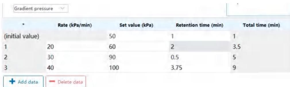
Figure 3-16 Gradient pressure edit interface
