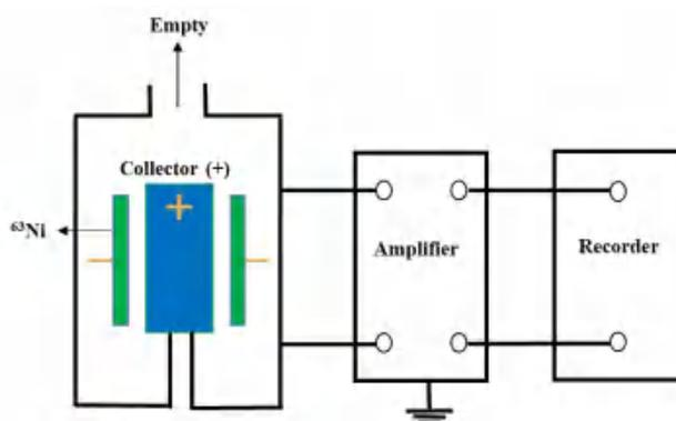
Figure1-10 Schematic diagram of ECD structure principle
