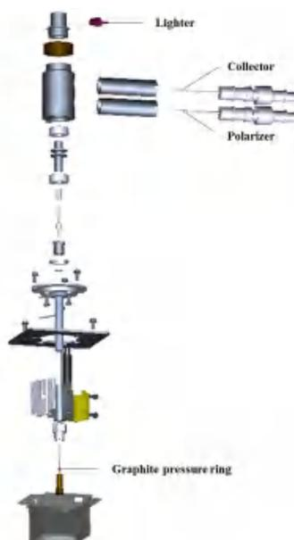
Figure 4-8 Schematic diagram of the structure of FID
