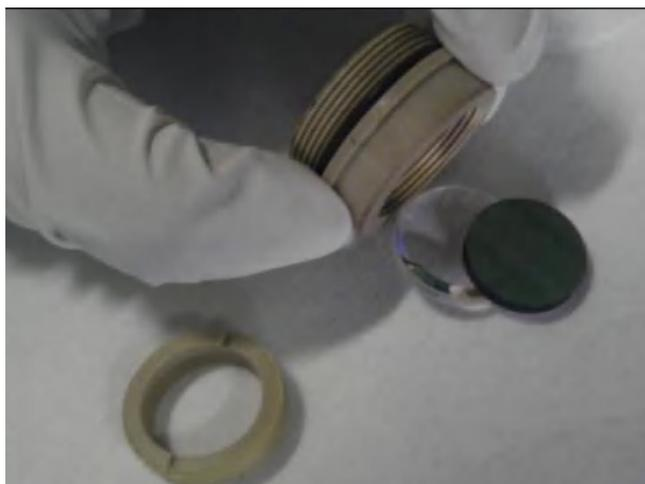
Figure 4-21 Remove the filter
