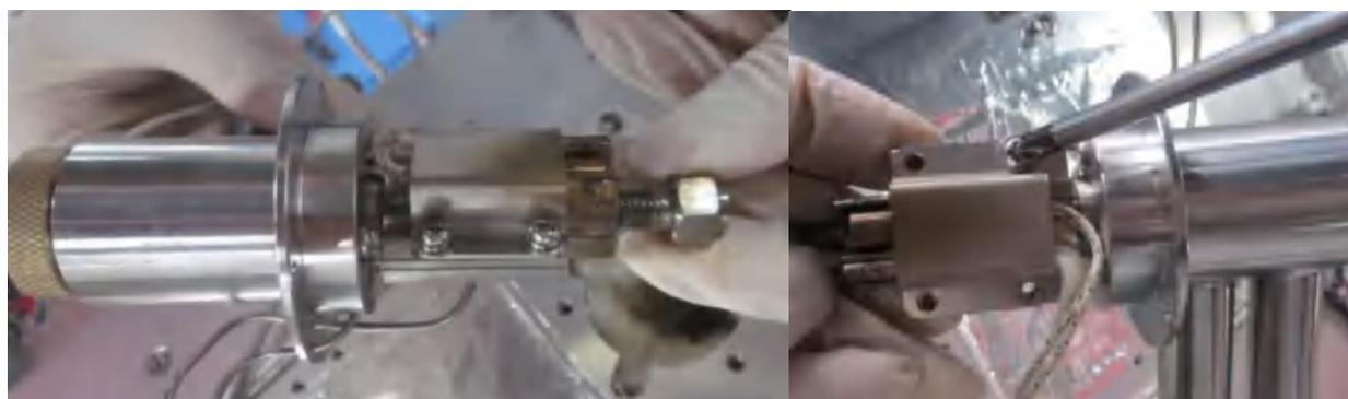
Figure 4-9 Take out the detector and remove the detector heating block
