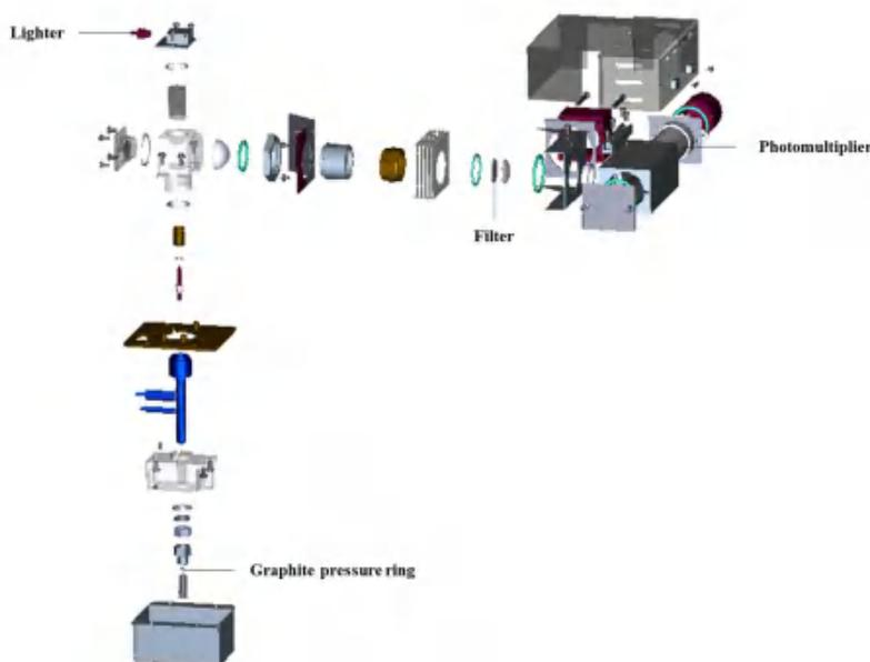
Figure 4-14 Schematic diagram of FPD structure
