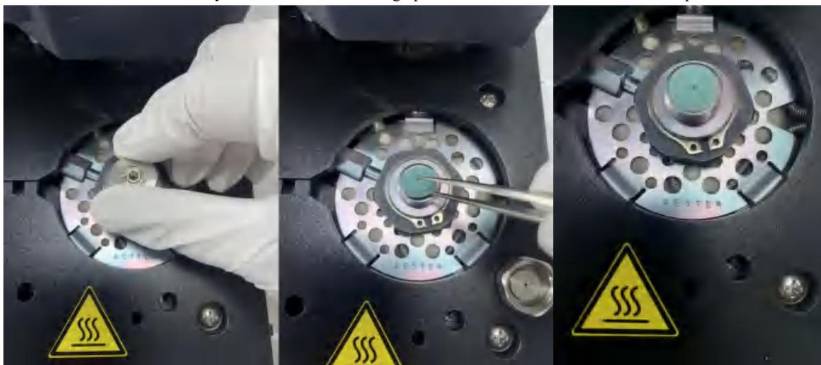
Figure 4-2 To replace the septum, users should unscrew the septum nut by hand, remove the septum with tweezers, and insert the new septum into the inlet
