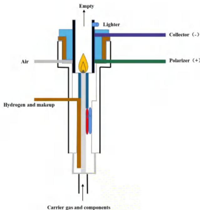
Figure1-7 Schematic diagram of the structure of FID
