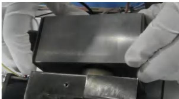
Figure 4-18 Remove the PMT outer sleeve
