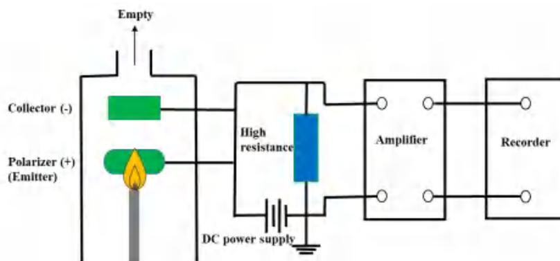
Figure1-8 Schematic diagram of FID structure principle
