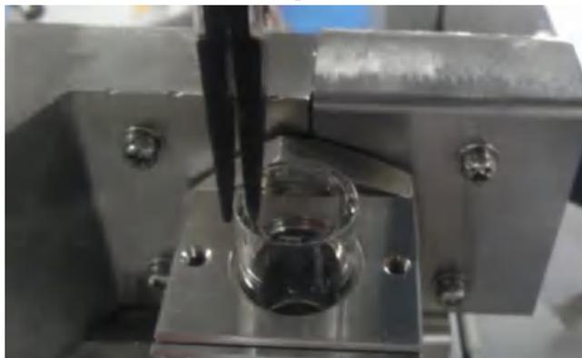
Figure 4-17 Take out the quartz sleeve
