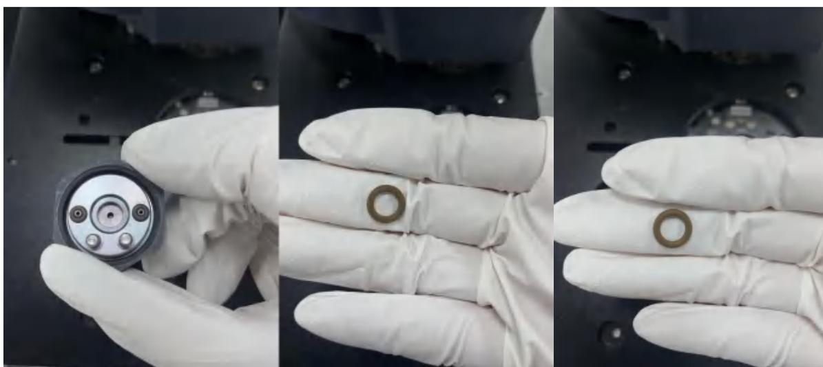
Figure 4-4 To replace the sealing ring, users should check two sealing rings 1, damaged sealing ring 2, and intact sealing ring 2
