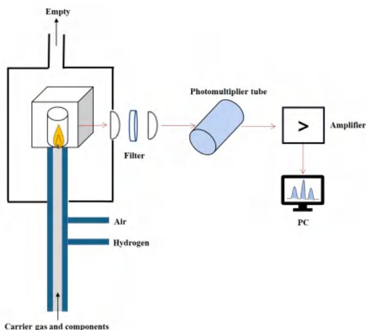
Figure1-11 Schematic diagram of FPD structure
