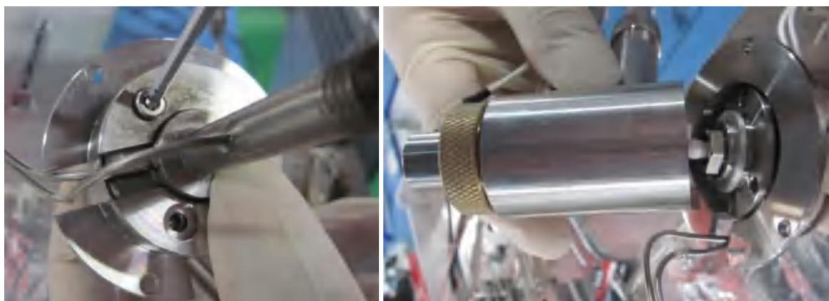
Figure 4-10 Remove the detector housing
