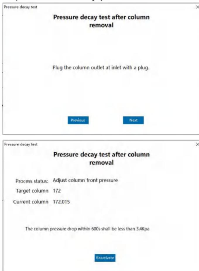
Figure 3-35 Pressure decay test window
