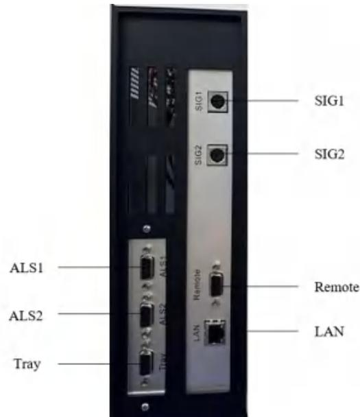
Figure1-5 Electronic cable interface
