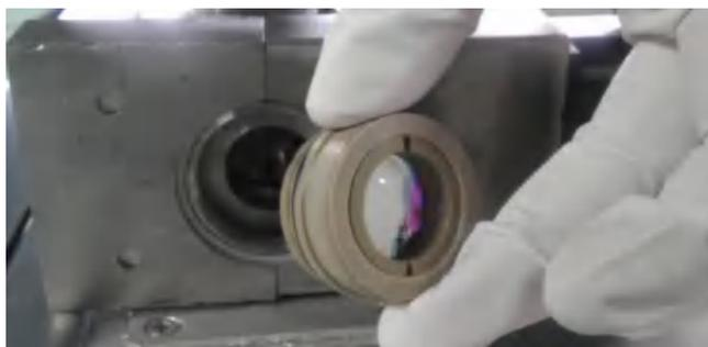
Figure 4-20 Remove the filter assembly
