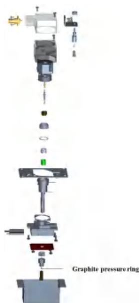
Figure 4-13 Schematic diagram of ECD structure
