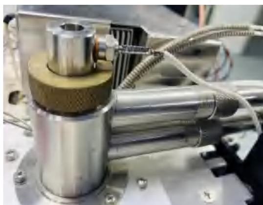
Figure 4-12 Ignition wire assembly
