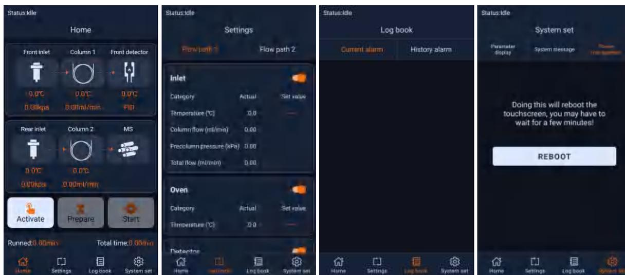
Figure 3-1 Touch screen interface (main interface, method setup, logging and system setup)
