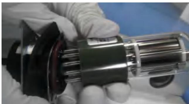
Figure 4-24 Replace the Photomultiplier Tube
