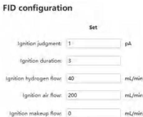
Figure 3-27 FID configuration window
