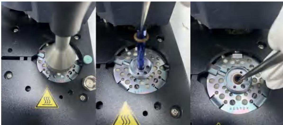
Figure 4-3 To replace the liner, users should unscrew the flow adapter block with a socket wrench, remove the liner with tweezers, place a new liner in the inlet, and push on the bottom
