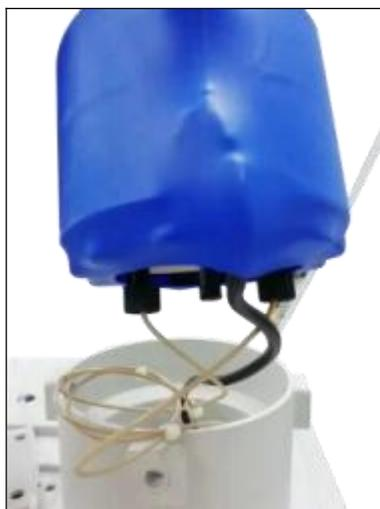
Figure 5-7 Pipeline connection of eluent generation tank
