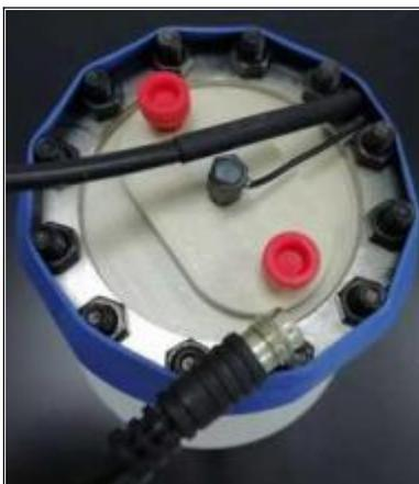
Figure 5-8 Plugs and cable of eluent generation tank
