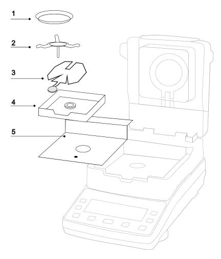
Please installation the instrument according the picture Installation order from top to bottom: 1 --2--3--4--5
