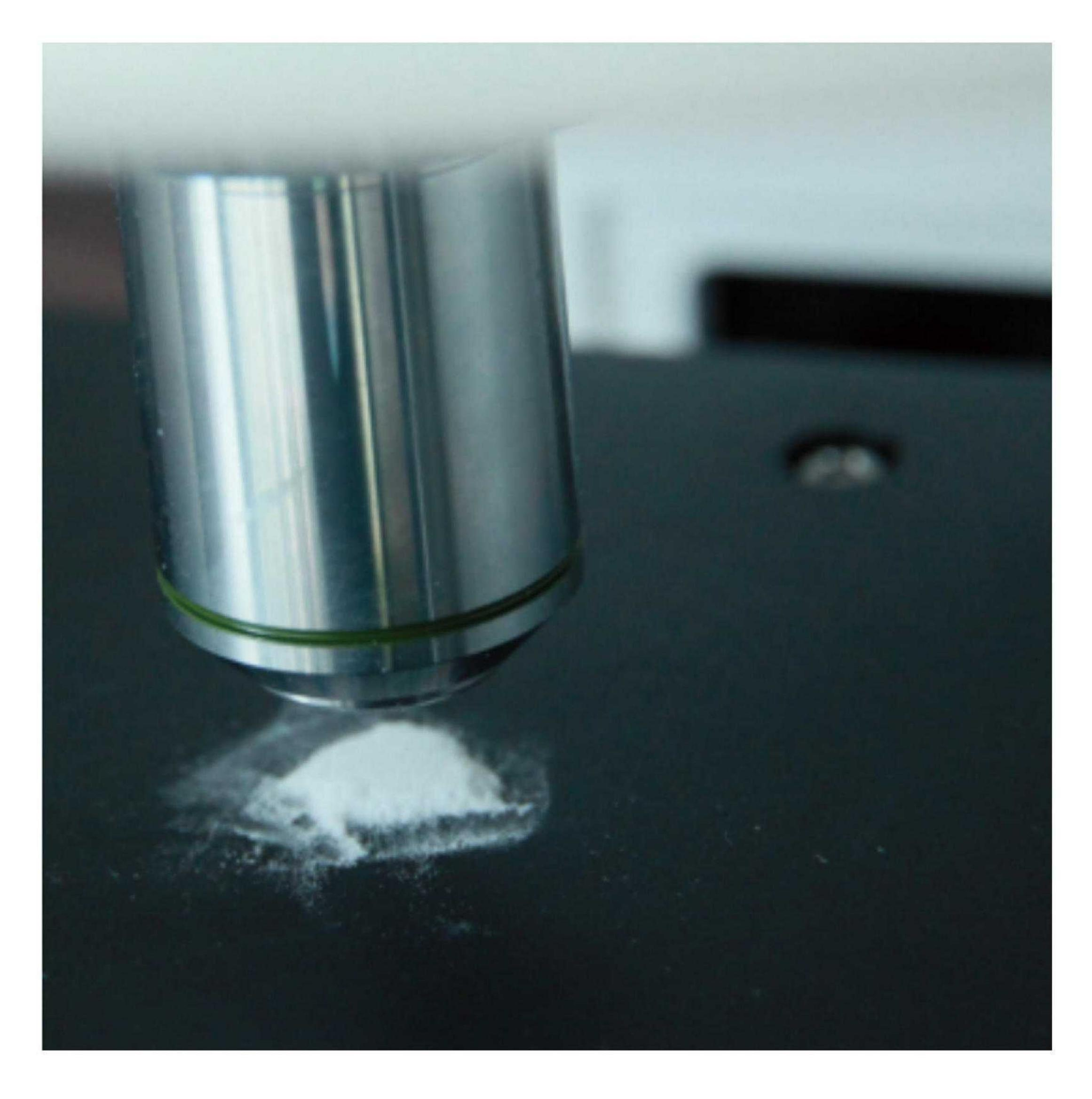
Fig 15 Raman signal high throughput objective, focal length reach up to 8 mm;
