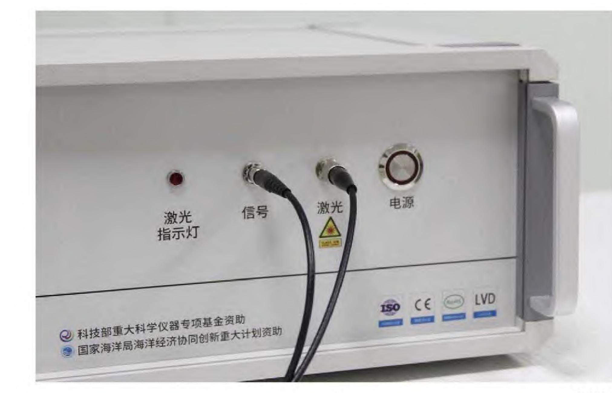
Fig 10 Power button, button on/off as many asl,000,000 times, high strength laser cable, signal cable is verystrong, and laser indicator can intuitively display operating status.
