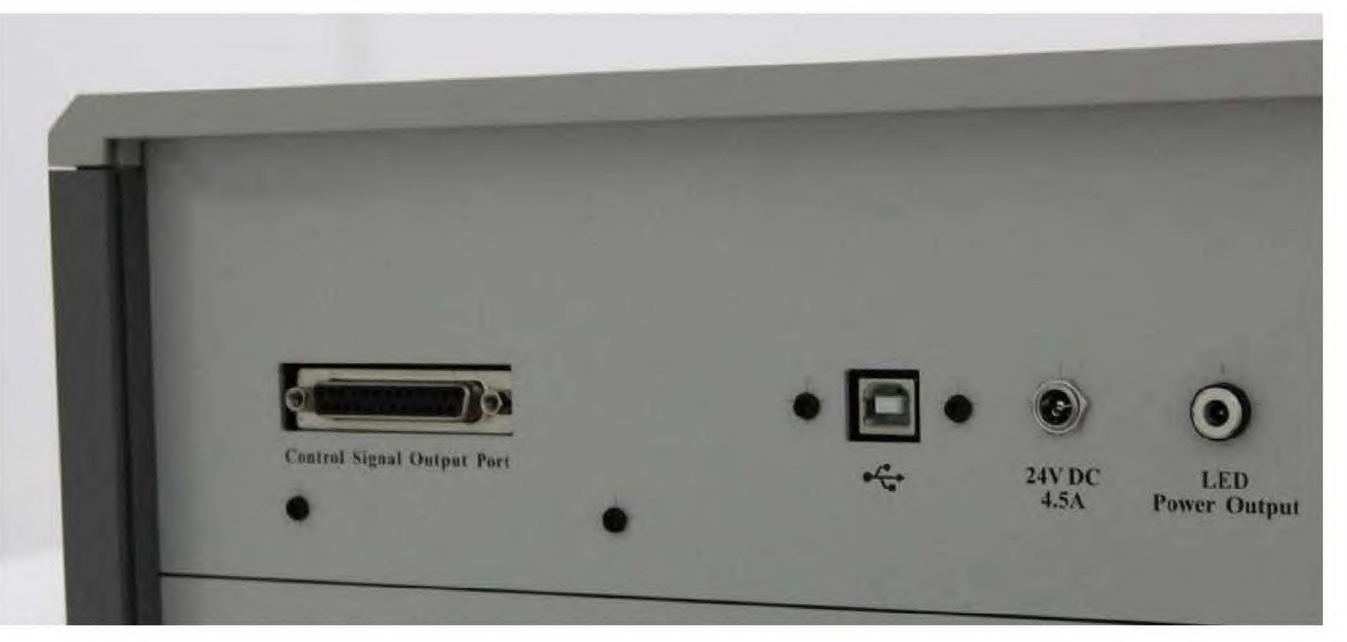
Fig 11 Simple interface: Raman spectrometer: power socket +USB2.0 connector
