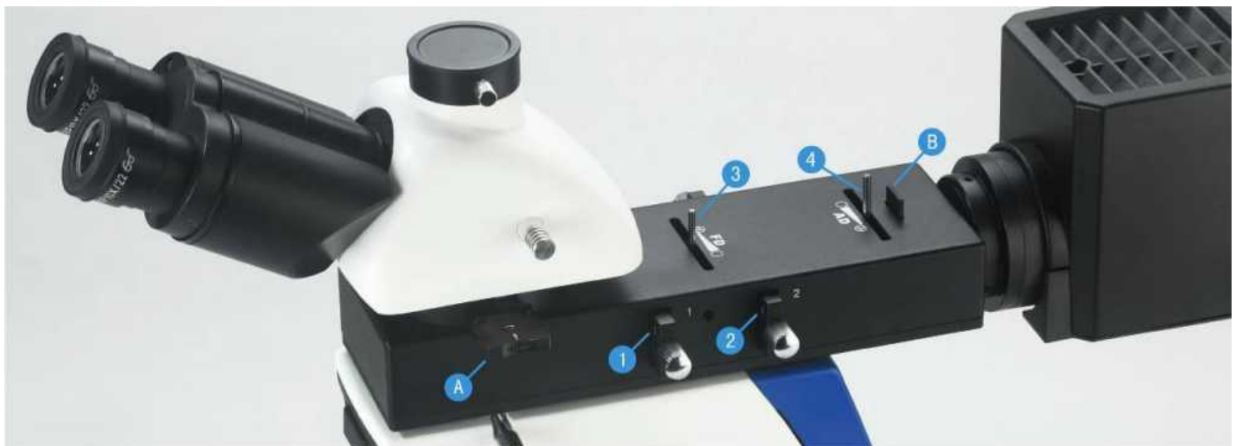
1. Polarizer 2.Filter switch handle 3. Field diaphragm 4.Aperture diaphragm A. Analyzer B. Ground glass slider
