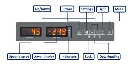
*MRF-40V368* Medical Combined Refrigerator and Freezer (upper 2~15°C and lower -40°C) is widely used in hospitals, blood stations and laboratories. The product has double chamber, double display, double control system, two sets of individual compressor and refrigeration system. Temperature in both chambers can be independently adjusted.
