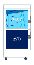
Rerigerator air-force circulation system keeps the chamber temperature flutuation externely stable at  $5\pm3^{\circ}$ C.
