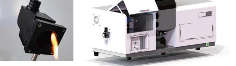
★ The new oxygen-enriched flame technology can be upgraded, and the flame temperature rises to above 2700°C, realizing a high-temperature flame without dangerous chemical laughing gas, and ensuring the determination of high-temperature elements Ca, Al, Ba, Mo, Ti, V, etc
