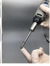
When assembling the dispersing tool, always make sure that the PTFE bearing is fixed correctly and cooled by the working medium. Otherwise, it may cause serious defects to the whole dispersing tool. Examine the PTFE bearings regularly. Treat the dispersing tools carefully as they are the hearts of your dispersing unit. In particular the axle reacts very sensitive to impacts.
