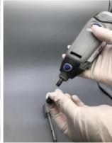
Remove collet nut and insert axle of the shaft into its place! Note: Please pull the Flexible collet (black) downward, ensure the shaft completely fixed.
