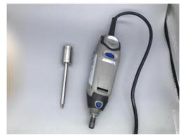
Hold HOMOGENIZER drive open the collet nut and press the blue button to unlock it and unscrew the collet nut
