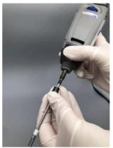
Put collet onto the shaft and screw it back to the drive itself! While doing that you must press the blue button to lock it
