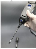
Put the shaft tube onto the axle and screw clockwise onto the housing! Press the blue locking button and screw it fully onto the drive!
